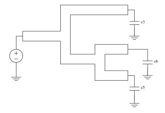
We divide the wires into 6 segments of fixed length  $l_i$ ; our variables will be the widths  $w_i$  of the segments. (The height of the wires is related to the particular IC technology process, and is fixed.) The total area used by the wires is, of course,
