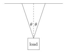
The (scalar) tensions  $T^{\text{left}}$  and  $T^{\text{right}}$  in the two cables are independently controllable, from 0 up to a given maximum tension  $T^{\text{max}}$ . The total force on the load is
